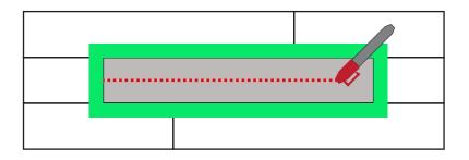
2. Mark out the center of the plank.
